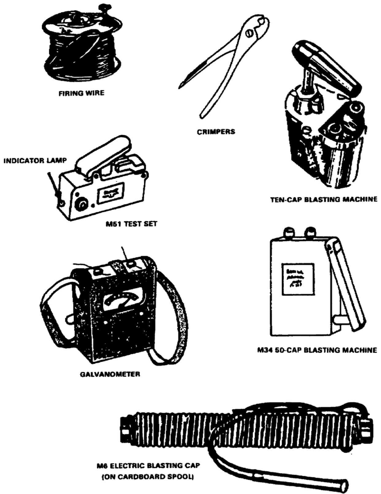
Figure 15. Electric firing system components and equipment.
